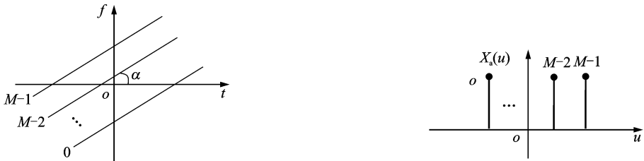
(a) 同距离单元不同横向距离散射点回波时频平面分布示意图 (a) Time-frequency plotting of scattered echo with different distance in same distance unit (b) 同距离单元不同横向距离散射点回波FrFT后分布示意图 (b) Distribution of scatter points of different distance in same distance range by FrFT
