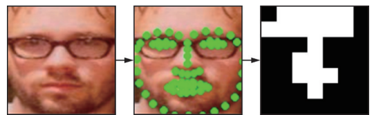
图2 基于关键部位掩码的注意力机制 Fig.2 Attention mechanism based on critical site masks
