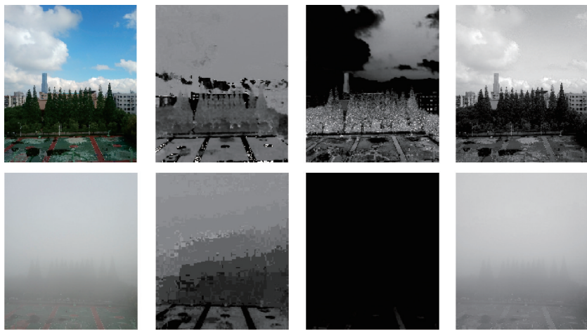
(a) Original images (b) Effect of H component (c) Effect of S component (d) Effect of V component
