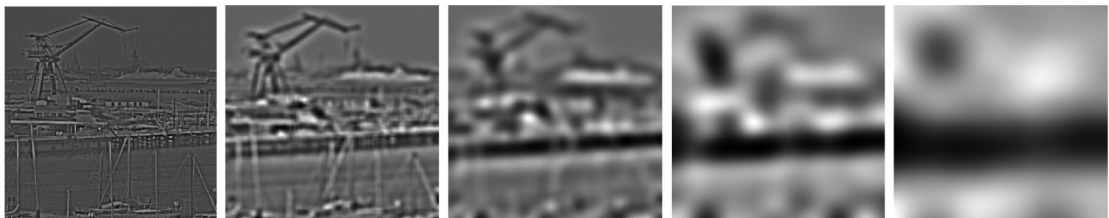
(a) IFABEMD方法分解的BIMF1~BIMF5分量 (a) BIMF1—BIMF5 results by IFABEMD method
