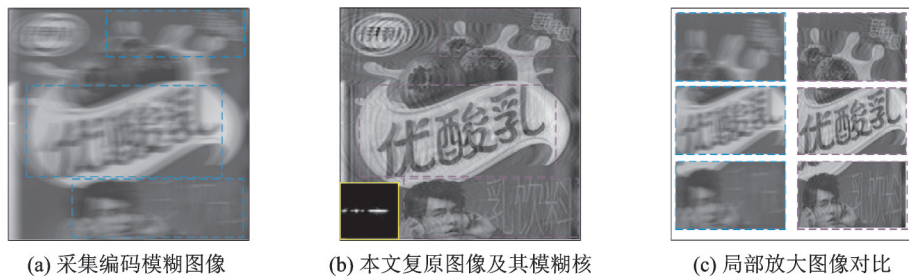
(a) 采集编码模糊图像 (b) 本文复原图像及其模糊核 (c) 局部放大图像对比 (a) Coded exposure blurred images (b) Restored image and its blurred kernel (c) Enlarged view of Figs.(a) and (b)
