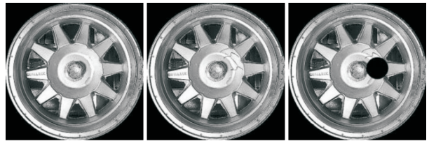
(a)正常轮毂图片 (a) Normal wheel (b)有文字污渍 (b) Wheel with characters stains (c)有明显缺陷 (c) Wheel with defect
