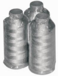
图 1 镀银导电纺线 Fig. 1 Silver-plated conductive thread
