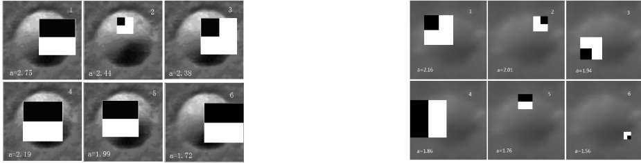
(a) 没经过阴影消除的撞击坑 (b) 经过阴影消除和属性形态学处理的撞击坑 (a) Crater without shadow elimination treatment (b) Crater after shadow elimination and attribute morphology
