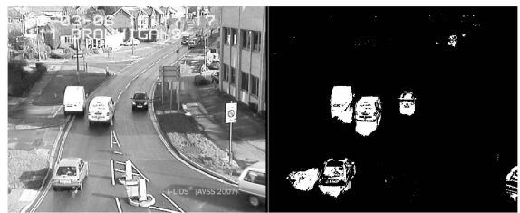
(b) 异常停车视频图像及检测后图像 (b) Abnormal park video image and image after detection
