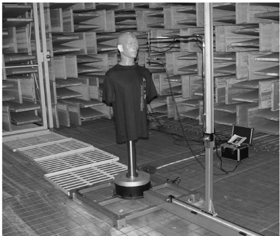
(a) 头和躯干相关传递函数的测量环境 (a) Environment for head and torso transfer function measurement
